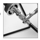
Attach the other end of the hose with the regulator to the gas cylinder, tightening using the two finger support posts.
